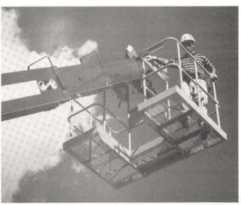
\*See service/parts bulletin #218 & #218A for allowable basket applications. \*Do not operate a Manitex crane or accessories within 10' (3.04M) of live power lines.
